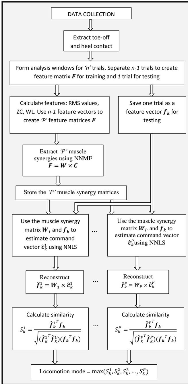
Fig. 1. Block diagram for the muscle synergy extraction algorithm
