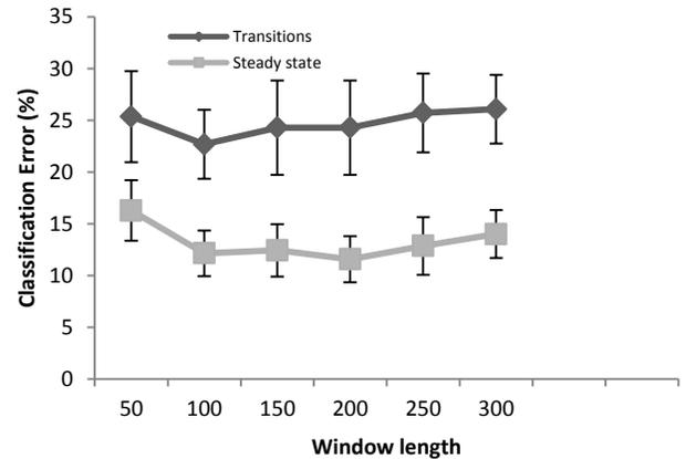
Fig. 3. Effect of analysis window size on classification error. Both the transitional and steady-state errors increased as the size of the analysis window increased. Significant increase in steady state error was observed for window size above 300 ms. Data are averages for seven subjects.
