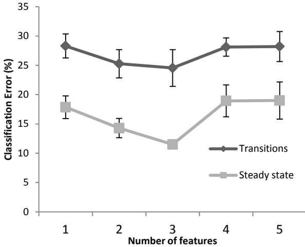
Fig. 4. Effect of number of features for extraction of muscle synergies. Three features produced the lowest transitional and steady state error.
