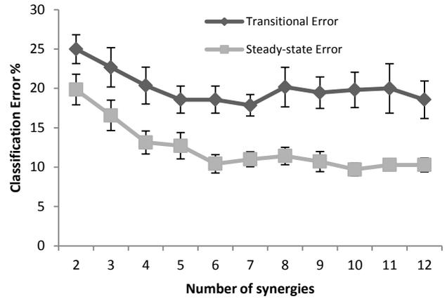
Fig. 2. Effect of the number of synergies on classification error. Both the transitional and steady-state errors decreased as the number of synergies was increased from 2 to 6. From 6 onwards the effect flattened. Data are averages for seven subjects.
