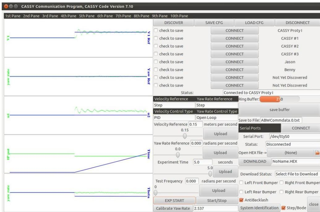
**Figure 4. Custom GUI (ABWComm4) to communicate with CASSY over Bluetooth.**
