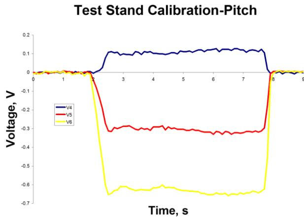
Figure 6 Response of legs 4-6 to simulated pitch.
