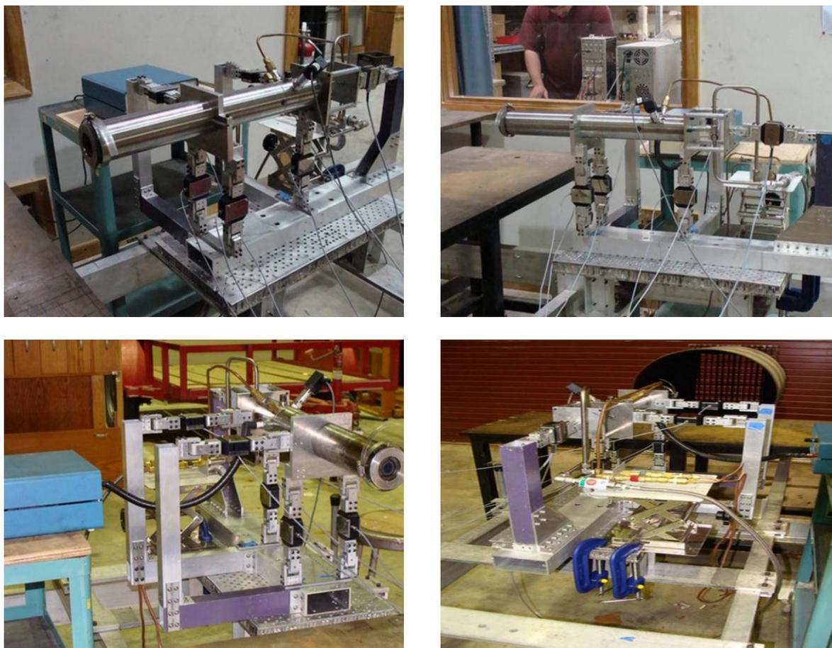
**Figure 4 The assembled thrust stand.**
