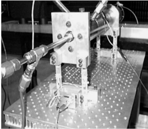
**Figure 1 Axial thrust measuring system, including strain gages mounted to four aluminum legs.**
