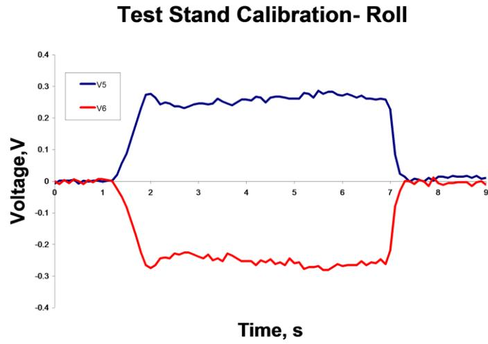
Figure 5 Response of legs 5 and 6 to simulated roll.
