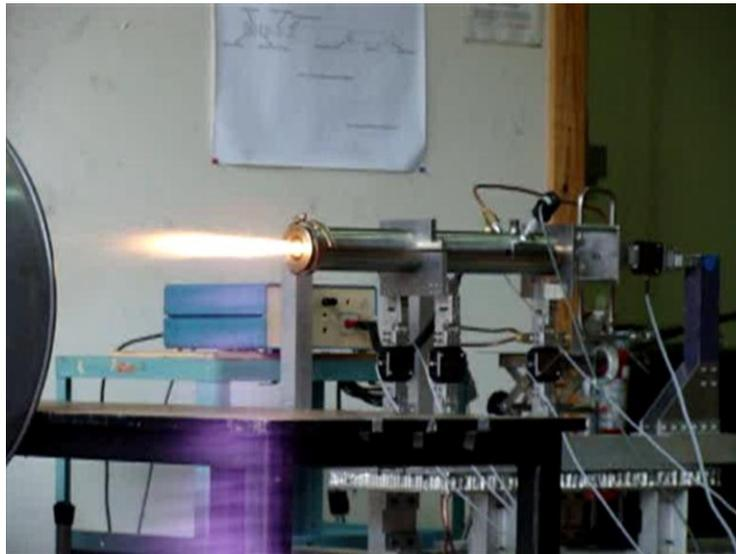
**Figure 8 The thrust stand remained stable during a rocket firing test.**
