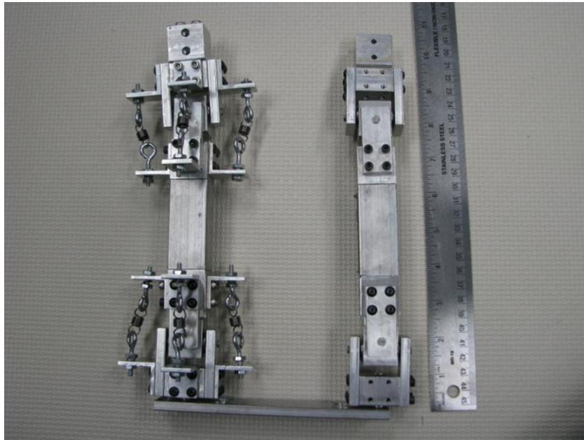
**Figure 3 Uniaxial leg with support springs (on left) and without springs (on right). The central block is a spacer for the load cell.**
