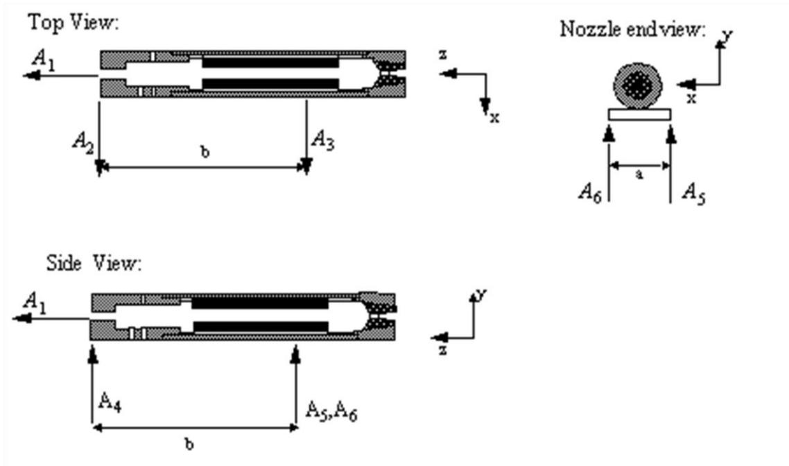
**Figure 2 Freebody Diagram of rocket body and six degree of freedom thrust sensor arrangement.**
