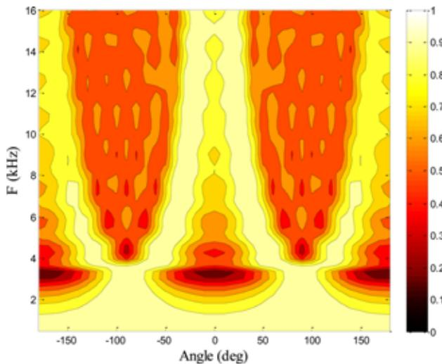
FIG. 7. (Color online) The directional response of the shotgun microphone simulated by the SWM.
