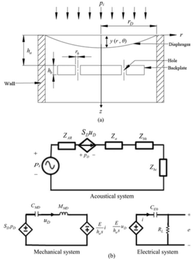
FIG. 1. Condenser microphone and the associated analogous circuits. (a) The cross section of a condenser microphone. (b) Electroacoustic analogous circuits.
