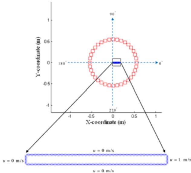
FIG. 8. (Color online) Schematic diagram for modeling diffraction effect using the ESM. (□, field points; ○, match points; ●, equivalent sources)
