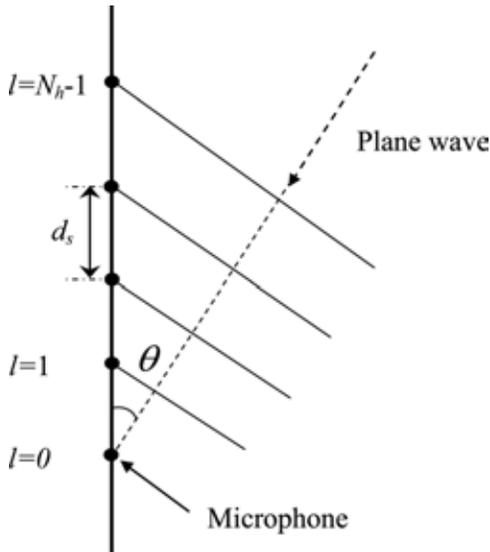
FIG. 2. Modeling the exterior field of a shotgun microphone from an array signal processing perspective.
