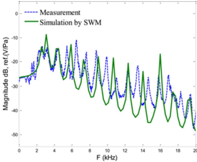
FIG. 6. (Color online) The on-axis frequency response of the shotgun microphone without mesh.
