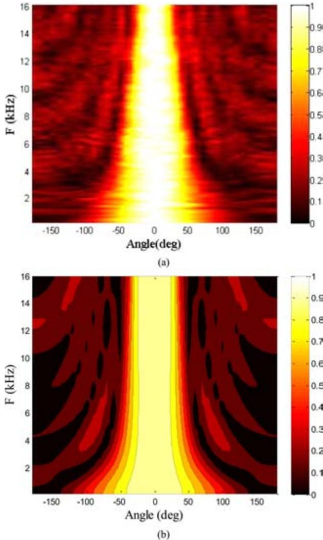
FIG. 12. (Color online) The directional responses of a commercial shotgun microphone (AT9913 of Audio-Technica). (a) Measurement, (b) Simulation based on the MSM.
