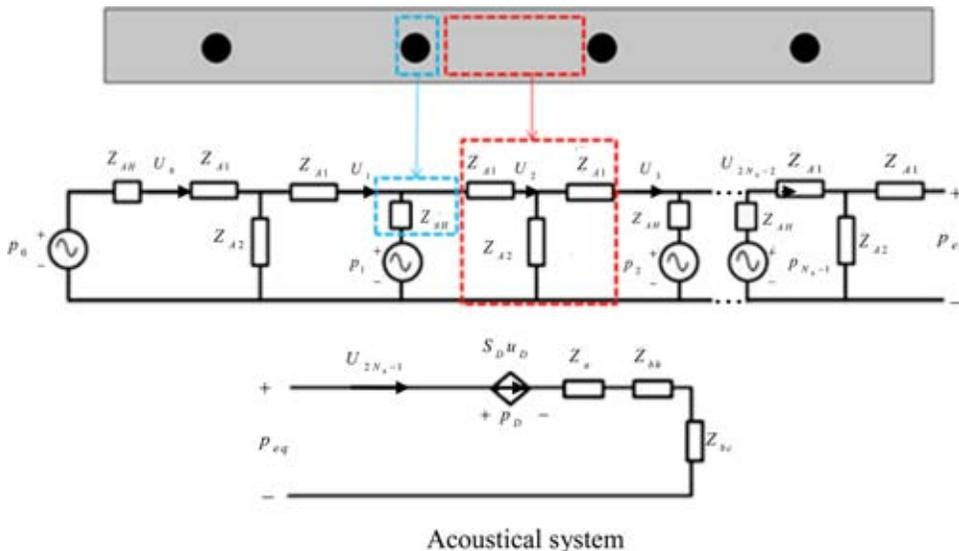
FIG. 5. (Color online) The SWM analogous circuits of the shotgun microphone, including acoustical, electrical, and mechanical domains.
