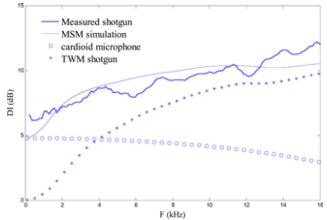
FIG. 13. (Color online) The directivity indexes plotted versus frequency of the shotgun microphone.
