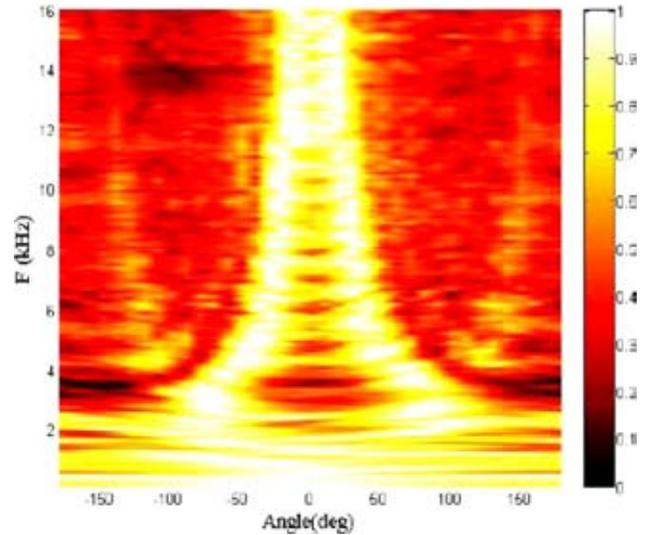
FIG. 4. (Color online) The measured directional response of a shotgun microphone with an omni-directional base element.
