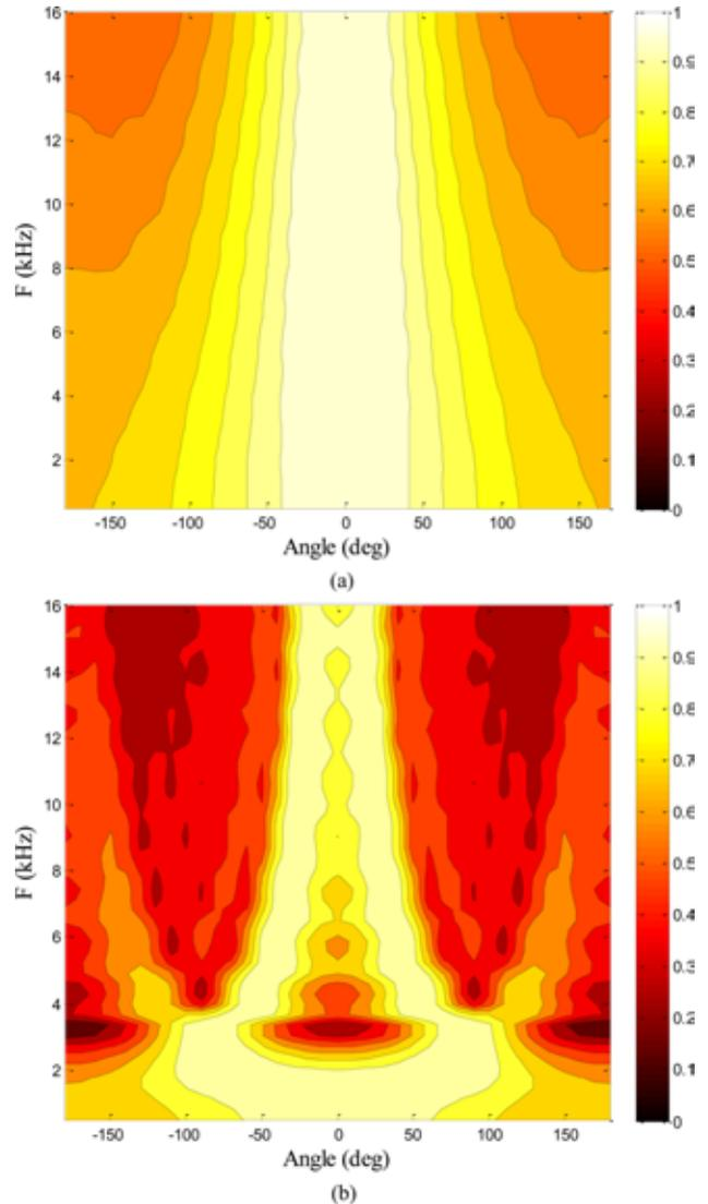
FIG. 9. (Color online) The directional response of the shotgun microphone with diffraction effect taken into account. (a) Diffraction pattern of the shotgun housing calculated by the ESM. (b) The combined directional response of the shotgun microphone simulated using the SWM and ESM.
