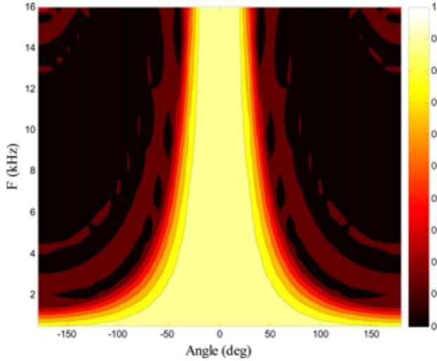
FIG. 3. (Color online) The directional response of a shotgun microphone simulated using the TWM.
